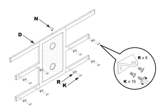
2-Fasten glass supporter (R) to the frames (D) with screws (K). Fasten glass protector (N) to the frames (D) .
